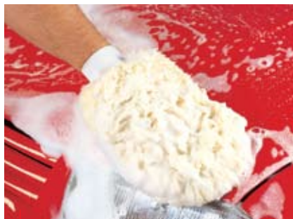
A Sheepskin Wash Mitt picks up a lot of dirt and distributes the cleaning agent evenly over the surface of the paint. Rinse your mitt often.
