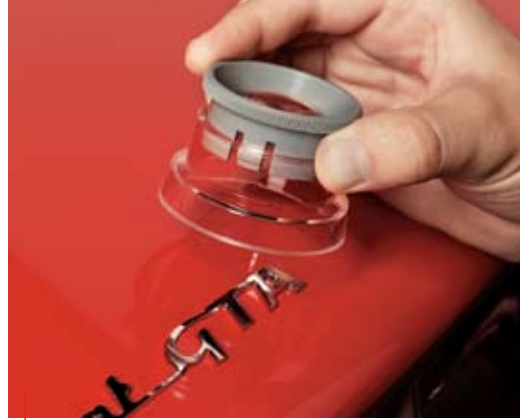
A Magnification Loupe makes it possible to see contaminants that are invisible with the naked eye.
