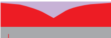
For deep scratches to be less noticeable, round off the "V" and "fill" the crevice with wax.
