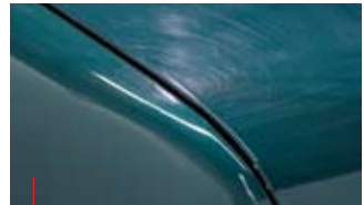
Swirl marks can be removed by polishing or hidden with several layers of Best of Show Wax.®
